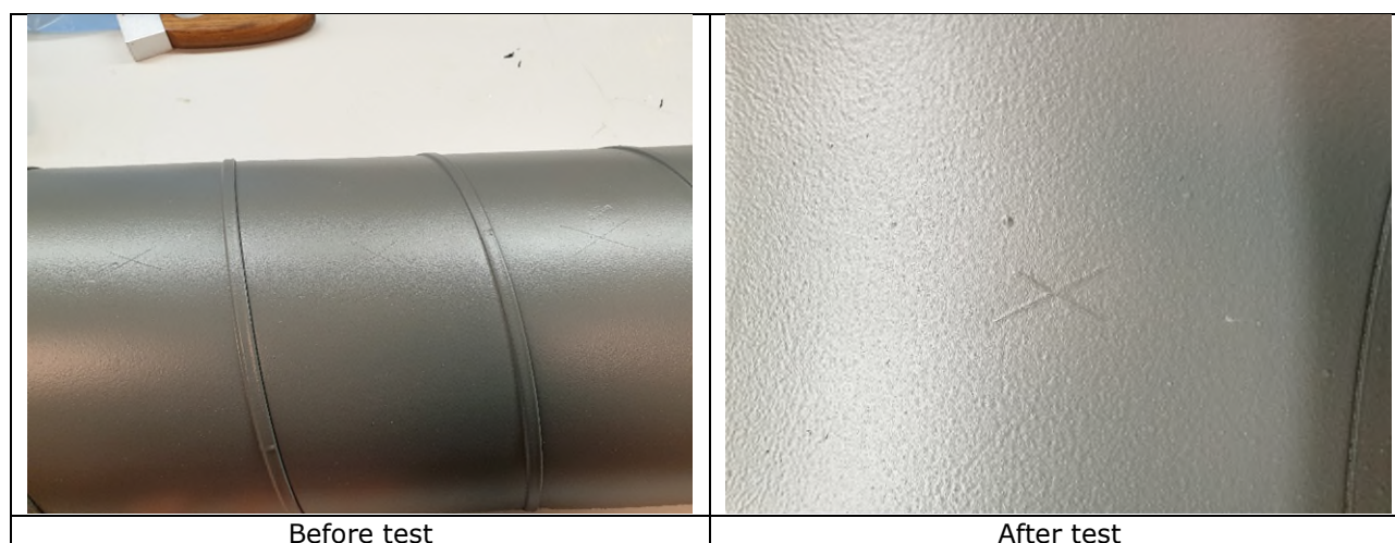
Figure 2: Test specimens before and after the adhesion test
