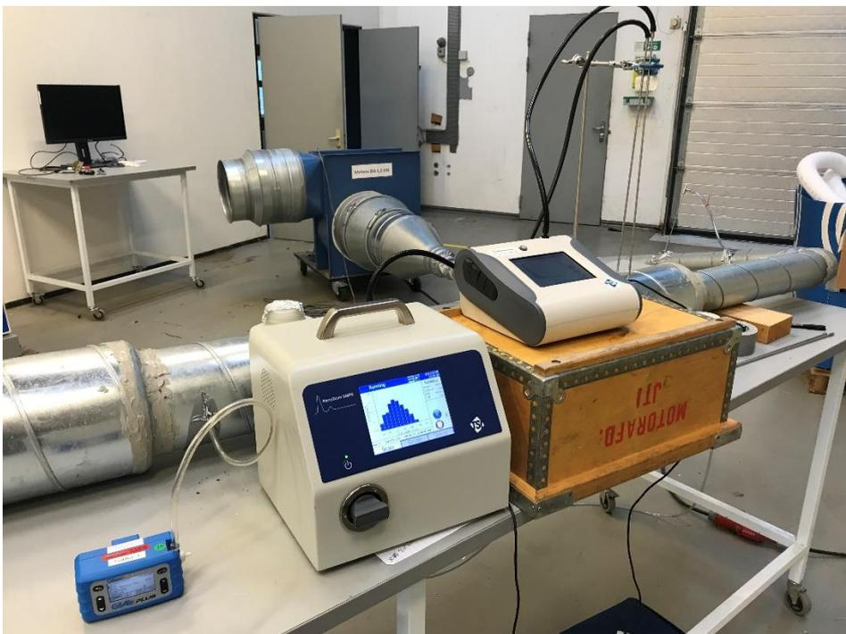
Figure 3: Measurements were performed in the  $\text{\O}160$  section with VOC to the left (most upstream) and the isokinetic sampling ports shown to the right (downstream).
