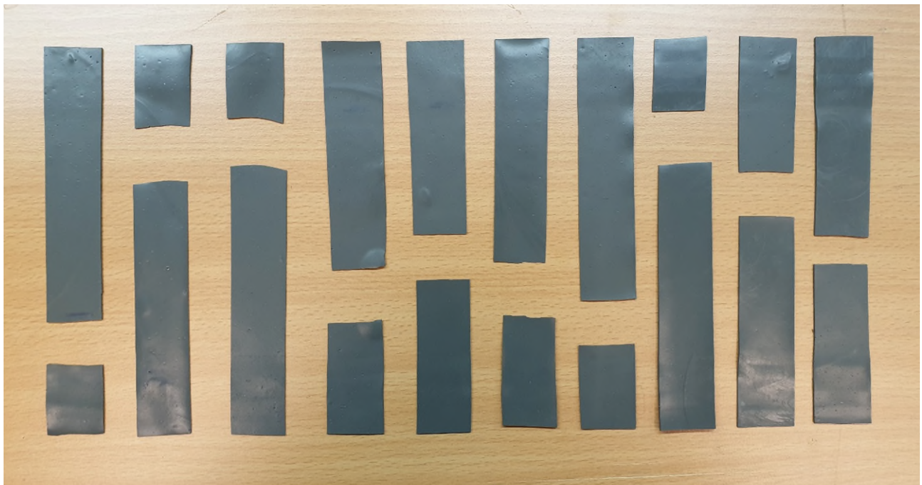
Figure 3: As prepared specimens after the tensile test
