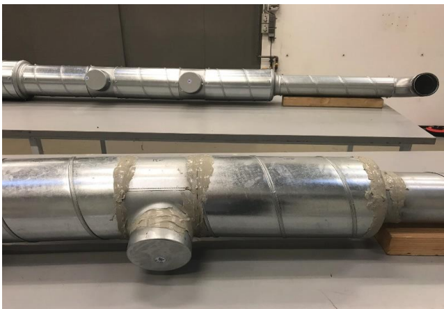
The joint sealant used to seal the duct joints outside
