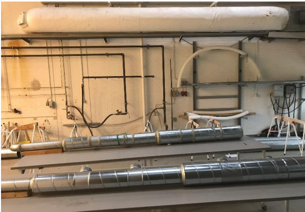
Pictures of the duct system with no coating and duct system with inner coating and joint sealant
