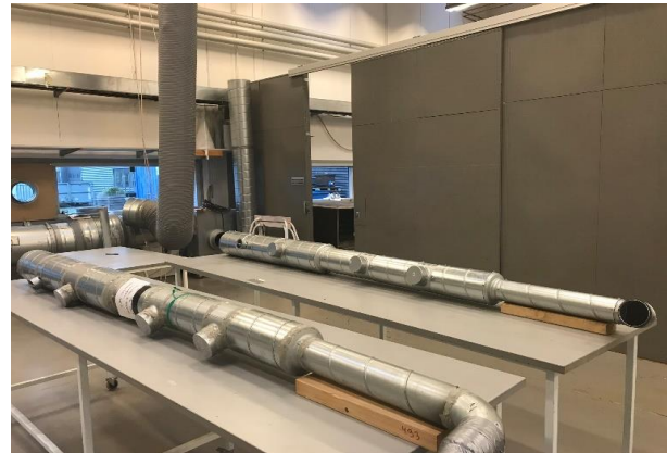
Pictures of the duct system with no coating and duct system with inner coating and joint sealant
