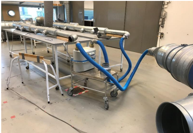
Picture of the leakage test setup
